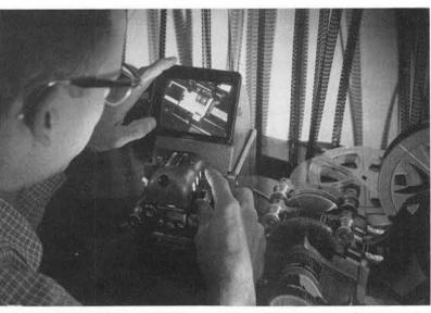
PAUL VAN DYKE (8123-3) uses film editor to view close-up of microfilm feed mechanism on a reproduction machine. Films Paul shot of the machine in operation revealed a malfunction in the machine and led to its correction by the manufacturing firm.
